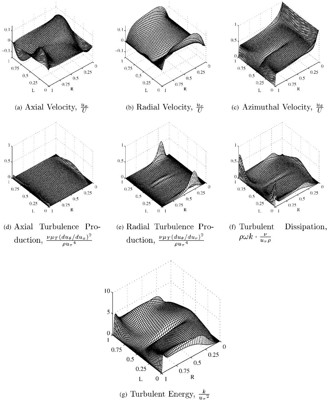
Figure 4. Components for square 48 mm case  $Re = 8 \times 10^3$ .
